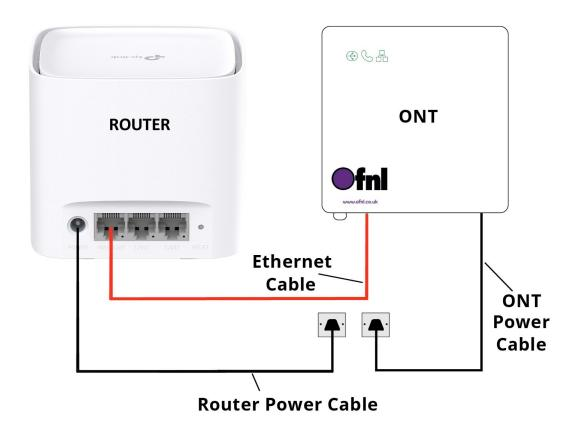
Please connect your router to the ONT (The ONT is often located in the hallway cupboard or under the stairs) using the ethernet cable provided (White or yellow cable included with your router).
